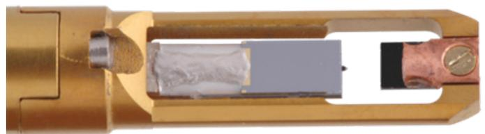
PI 95 TEM PicoIndenter front end showing MEMS transducer and sample mount.
